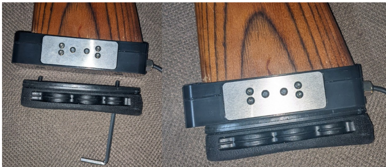
Figure 11: Recoil Pad Attached using 10-24 fasteners. Note fastener length protruding beyond the surface of the recoil pad is approximately 1/4". That is plenty of length to engage the threaded inserts in the Recoil-IQ. Screwing in longer screws could bottom out on the wood screw and destroy the Recoil-IQ.
