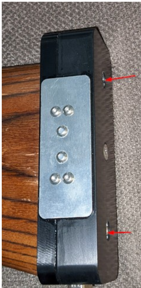
Figure 10 Threaded inserts installed until just recessed below surface.
