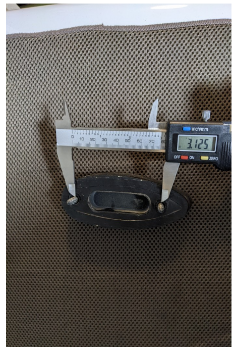
Figure 5: 3 1/8" buttplate hole spacing as shown on stock recoil pad removed from firearm.
