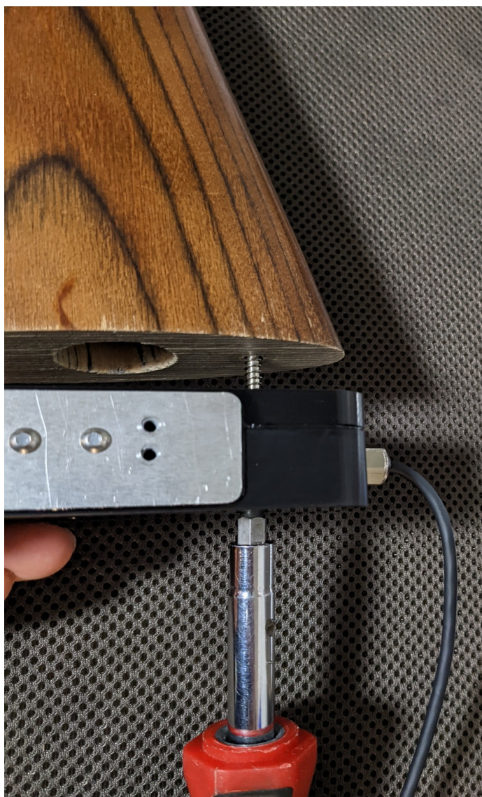
Figure 9: Hard Mount Screw Insertion
